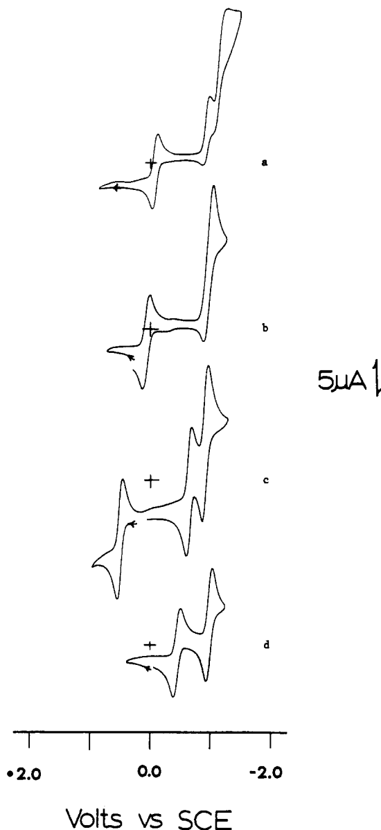
Figure 1. Cyclic voltammograms in 0.2 M TBAH-dichloromethane (at 200 mV/s with a Pt-bead electrode): (a) [(\eta^5\text{-C}_5\text{H}_5)_2\text{Co}][\text{Re}_2\text{Cl}_6(\text{PEt}_3)_2] ; (b) [(\eta^5\text{-C}_5\text{H}_5)_2\text{Co}][\text{Re}_2\text{Cl}_6(\text{PMePh}_2)_2] ; (c) [(\eta^5\text{-C}_5\text{H}_5)_2\text{Co}][\text{Re}_2\text{Cl}_5(\text{PMePh}_2)_3] ; (d) [(\eta^5\text{-C}_5\text{H}_5)_2\text{Co}][\text{Re}_2(\text{O}_2\text{CCMe}_3)_4\text{Cl}_2] .
